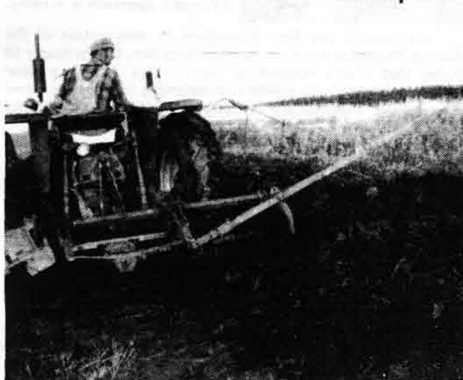
—Edgar Wuebben built his own compost turning machine entirely from old equipment on the farm. An old tool bar, gear box, and silage auger make the major components. The auger on the right opens up the compost windrow, aerating the material. Later a front-end loader repiles the windrow.
